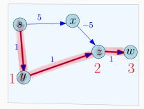
With negative length edges, Dijkstra's algorithm can fail.
