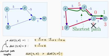
With negative length edges, Dijkstra's algorithm can fail.
