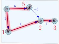
Dijkstra's algorithm terminates with  $d(s,z)=2:s\xrightarrow{t} y\xrightarrow{t} z$ . But the shortest path length is  $0:s\xrightarrow{5} x\xrightarrow{-5} z$ .
