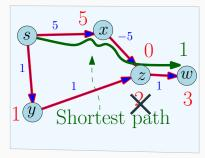
False assumption: Dijkstra's algorithm is based on the assumption that if  $s \to v_0 \to v_1 \to v_2 \dots \to v_k$  is a shortest path from s to  $v_k$  then  $dist(s, v_i) \le dist(s, v_{i+1})$  for  $0 \le i < k$ . Holds true only for non-negative edge lengths.
